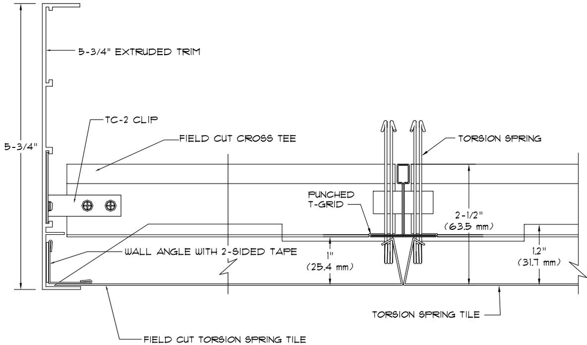
SECTION - FIELD CUT TORSION SPRING PANEL WITH 5-3/4" EXTRUDED PERIMETER TRIM
