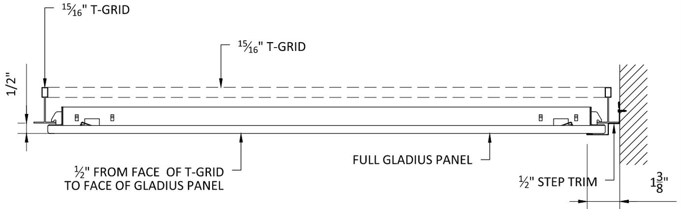
TYPICAL PERIMETER SECTION - full panel at wall angle
