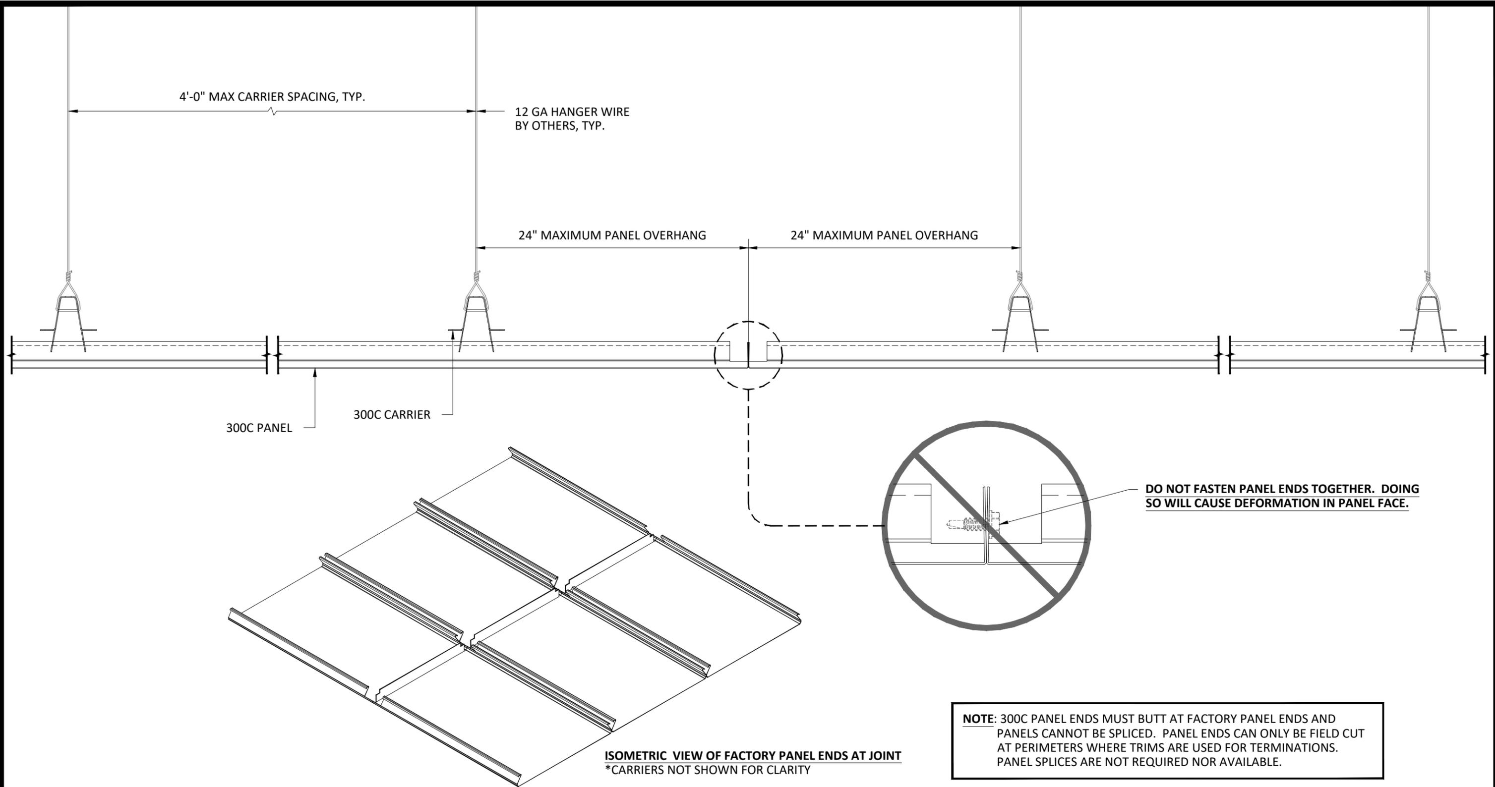
**DO NOT FASTEN PANEL ENDS TOGETHER. DOING SO WILL CAUSE DEFORMATION IN PANEL FACE.**
