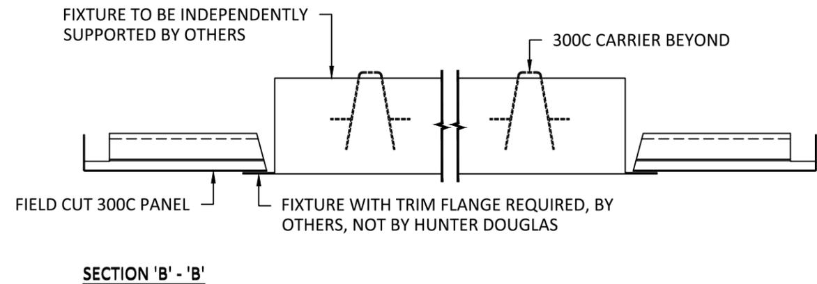
**NOTE:** ROUND OPENINGS LESS THAN EIGHT (8) INCHES DIAMETER TYPICALLY FIELD CUT INTO PANEL FACE, TRIM FOR ALL FIXTURES BY OTHERS NOT BY HUNTER DOUGLAS
