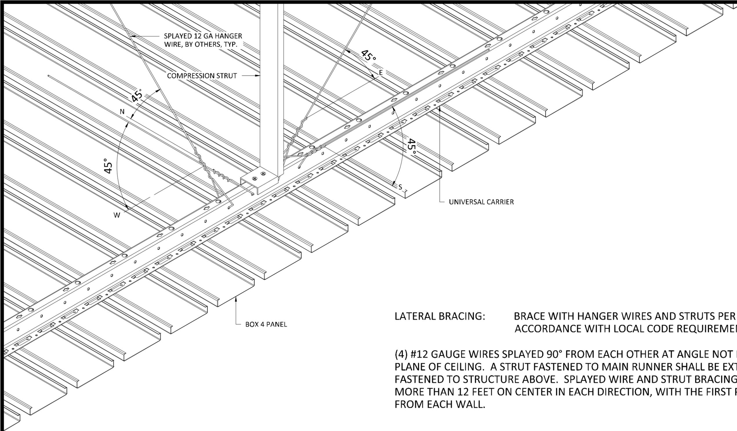
**LATERAL BRACING:** BRACE WITH HANGER WIRES AND STRUTS PER ASTM E-580 AND IN ACCORDANCE WITH LOCAL CODE REQUIREMENTS.
