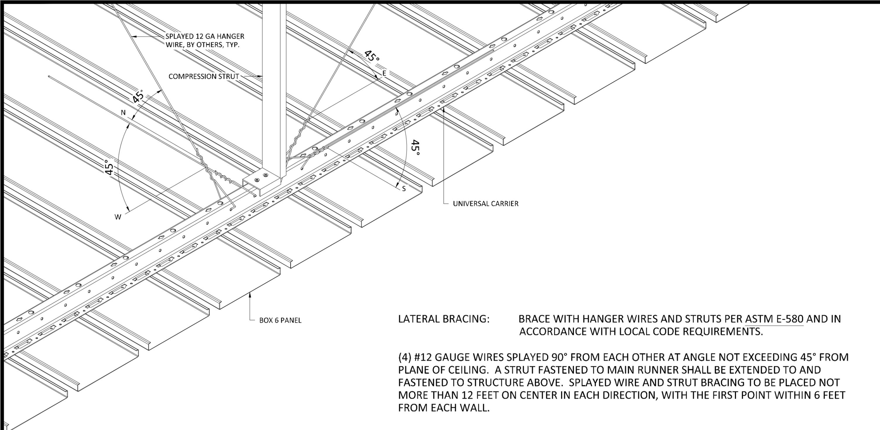
**LATERAL BRACING:** BRACE WITH HANGER WIRES AND STRUTS PER ASTM E-580 AND IN ACCORDANCE WITH LOCAL CODE REQUIREMENTS.
