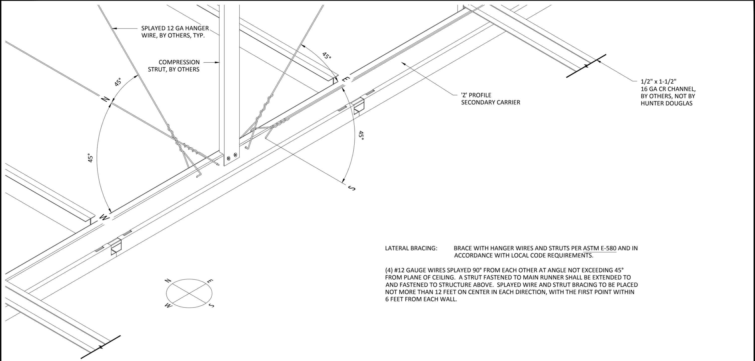
LATERAL BRACING: BRACE WITH HANGER WIRES AND STRUTS PER ASTM E-580 AND IN ACCORDANCE WITH LOCAL CODE REQUIREMENTS.
