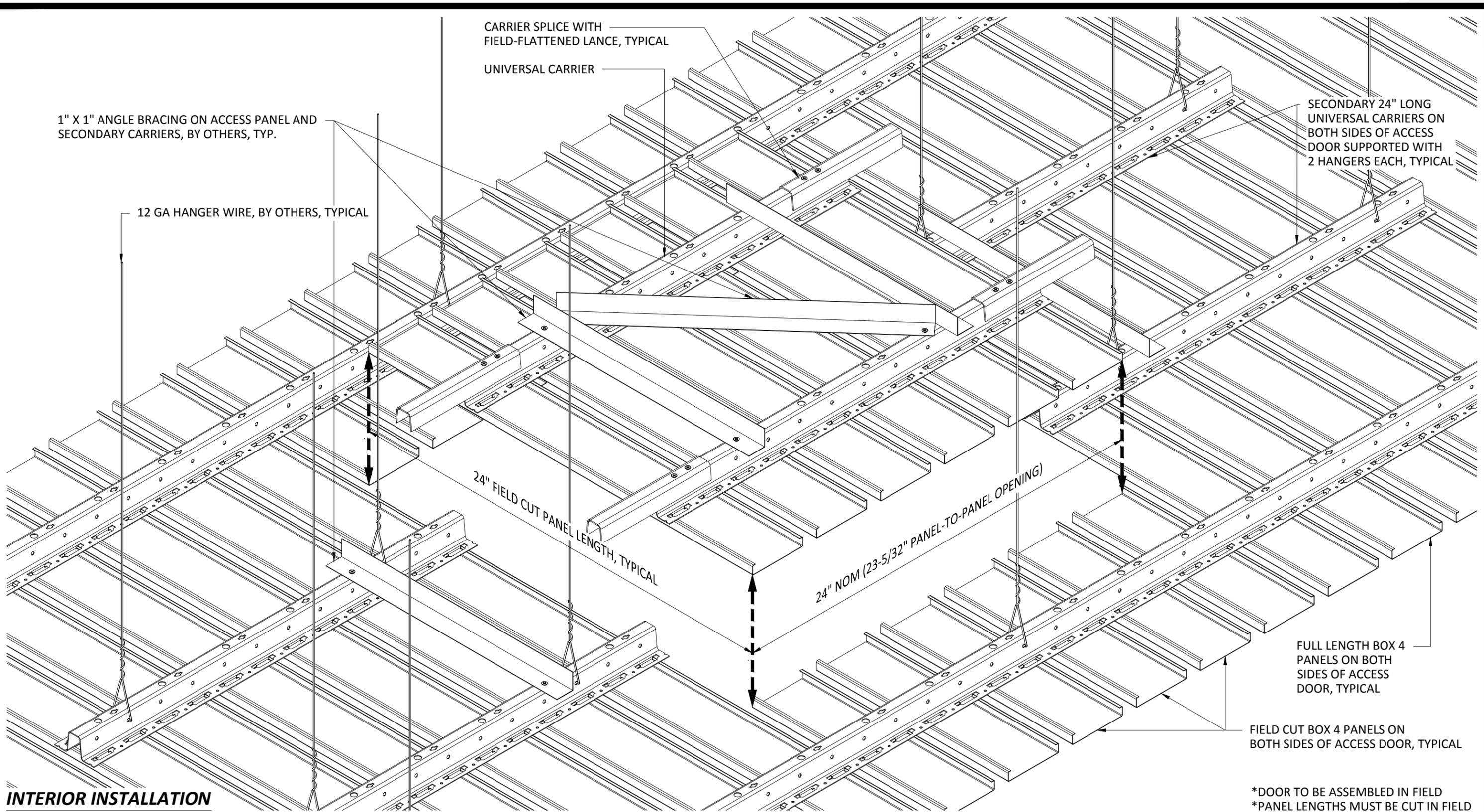
1" X 1" ANGLE BRACING ON ACCESS PANEL AND SECONDARY CARRIERS, BY OTHERS, TYP.
