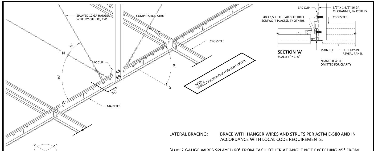
(4) #12 GAUGE WIRES SPLAYED 90° FROM EACH OTHER AT ANGLE NOT EXCEEDING 45° FROM PLANE OF CEILING. A STRUT FASTENED TO MAIN RUNNER SHALL BE EXTENDED TO AND FASTENED TO STRUCTURE ABOVE. SPLAYED WIRE AND STRUT BRACING TO BE PLACED NOT MORE THAN 12 FEET ON CENTER IN EACH DIRECTION, WITH THE FIRST POINT WITHIN 6 FEET FROM EACH WALL.
