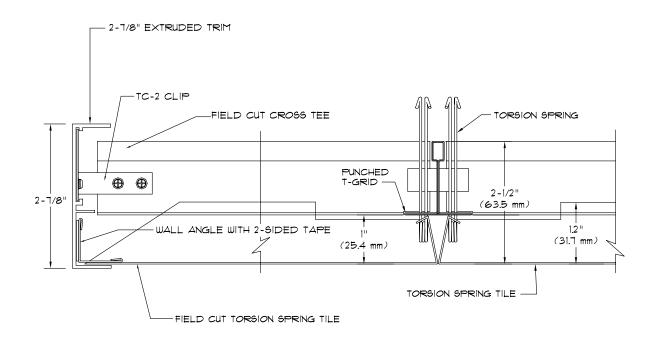
SECTION - FIELD CUT TORSION SPRING PANEL WITH 2-1/8" EXTRUDED PERIMETER TRIM
