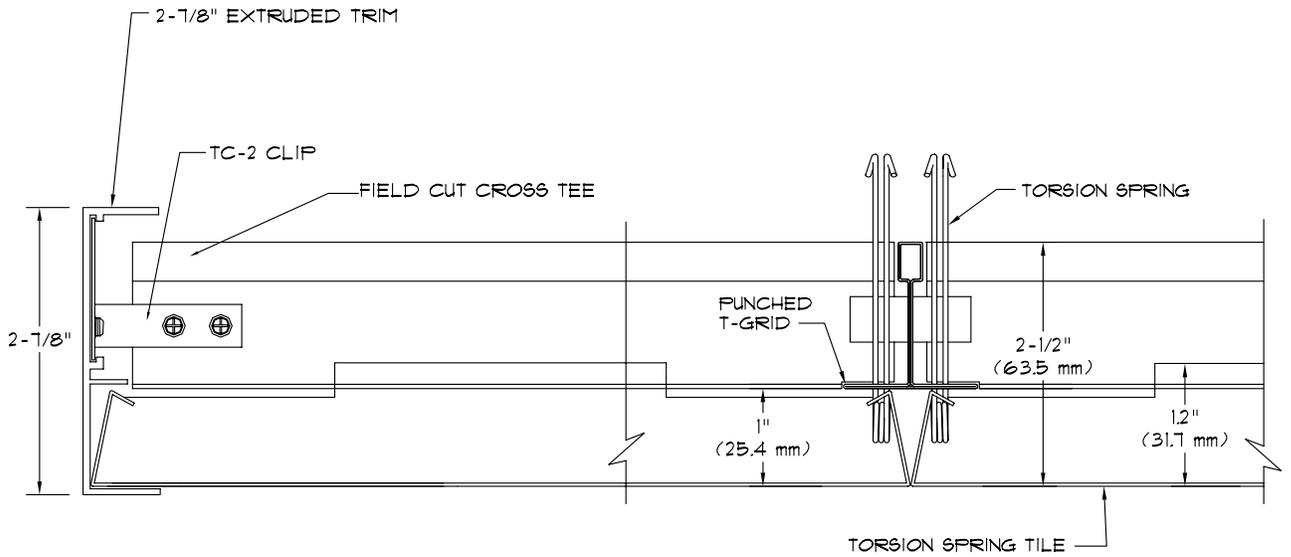
SECTION - FULL TORSION SPRING PANEL WITH 2-7/8" EXTRUDED PERIMETER TRIM
