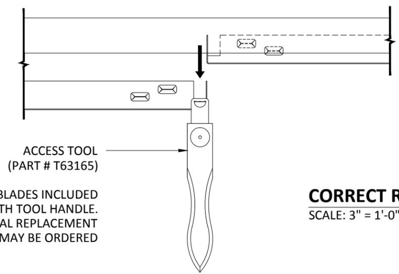
TO FIND CORRECT LOCATION FOR ACCESS TOOL, INSERT ACCESS TOOL AT PANEL INTERSECTION. ALIGN EDGE OF BLADE WITH EDGE OF PANEL. IF INSERTED IN PROPER LOCATION, YOU SHOULD HEAR A "CLICK" SOUND AND THE WOODEN HANDLE WILL SEAT FLUSH AGAINST THE PANEL FACE. IF NOT INSERTED IN PROPER LOCATION, BLADE WILL STOP BEFORE WOOD HANDLE SEATS. IF THIS HAPPENS, REMOVE TOOL AND INSERT IN ADJACENT PANEL EDGE. (AROUND THE CORNER).
