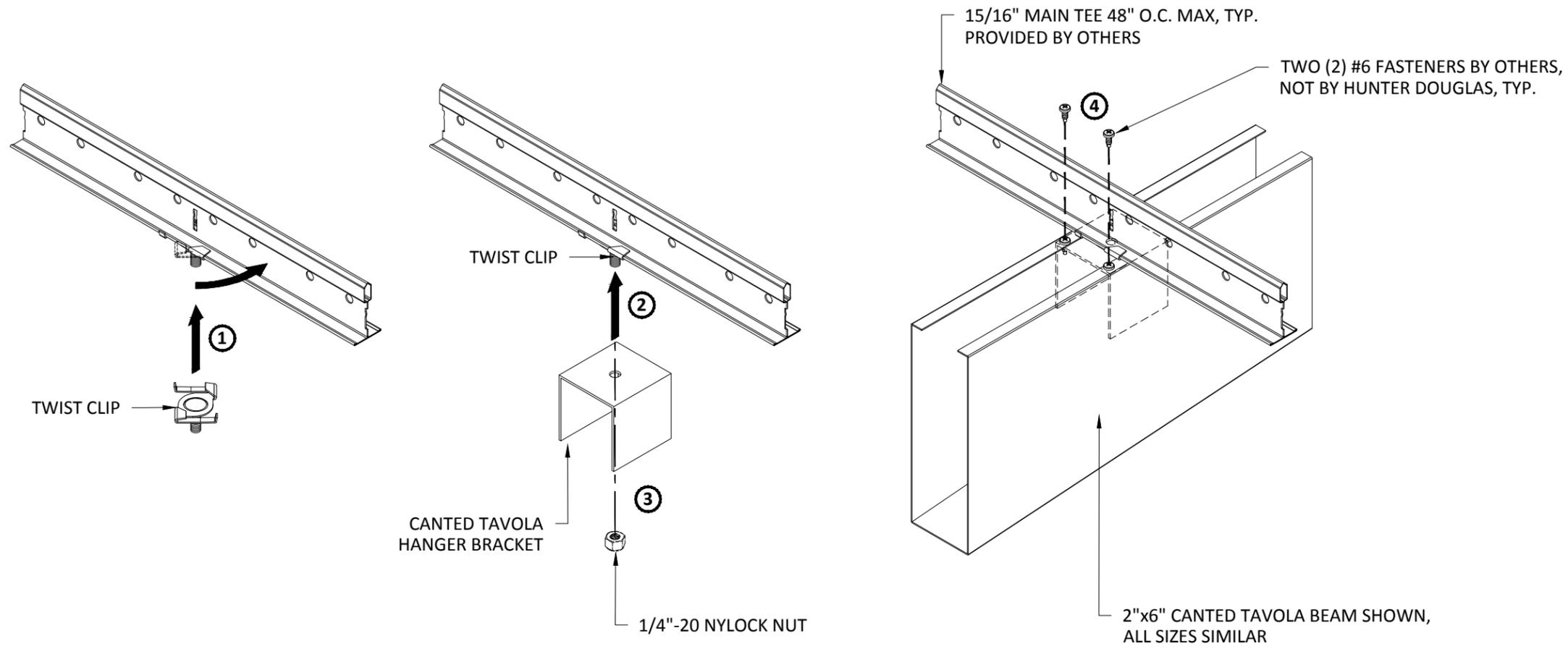
① INSERT TWIST CLIP ONTO MAIN TEE AND ROTATE INTO POSITION
