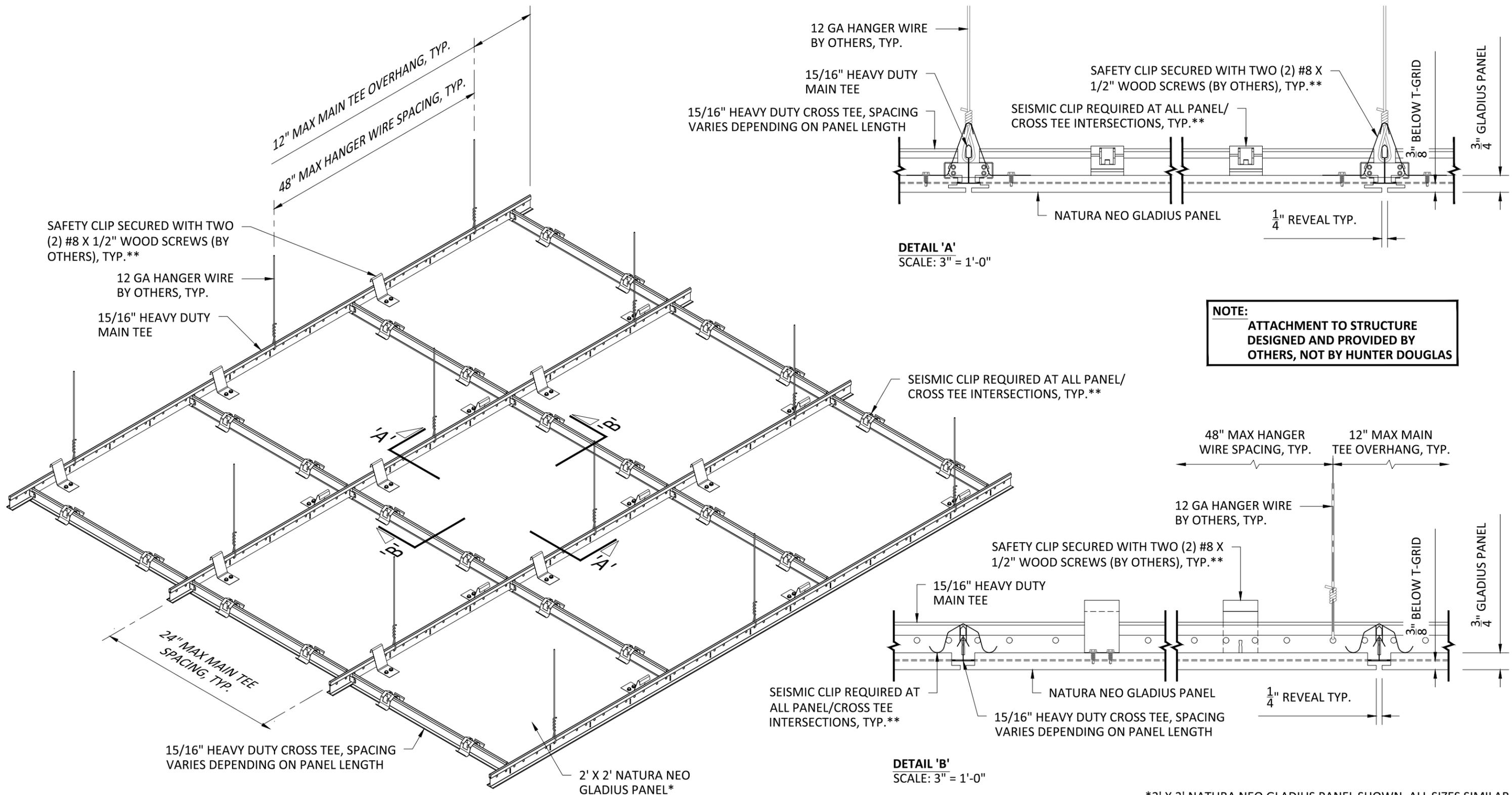
SAFETY CLIP SECURED WITH TWO (2) #8 X 1/2" WOOD SCREWS (BY OTHERS), TYP.\*\*
